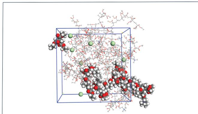
**Fig. 1:** Simulation box (3.4 x 3.4 x 3.4 nm) with periodic boundaries showing 8 Eudragit® RS polymer chains and 2 TEC plasticizer molecules after a relaxation time of 2 ns at 460 K. One polymer chain and one TEC molecule are visualized in ball and stick style to demonstrate the size of the box in relation to the coiled polymer chain.
